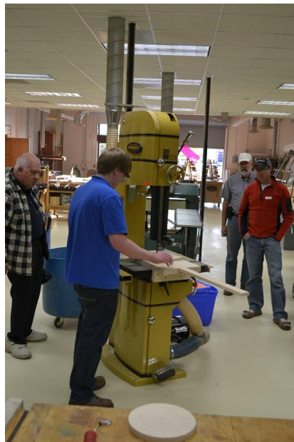
Ben King demonstrated a circle cutter that he made for cutting bowl blanks on a band saw.
